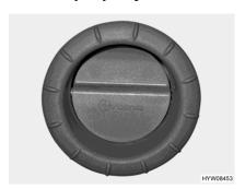
Fig. 103 Air outlet nozzle (hot-air heater)
