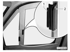
Fig. 26 Roman shade (driver's / front passenger's window, Mercedes-Benz)
