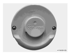
Fig. 114 Wall flue (hot-air heater)
