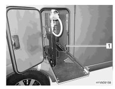
Fig. 82 Gas bottle compartment pull-out in changing position
