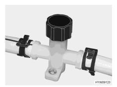
Fig. 112 Safety/drainage valve (boiler)
