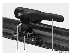
Fig. 21 Catch lever ("continuous ventilation" position)
