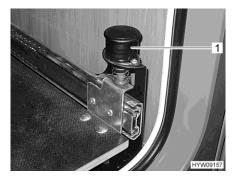
Fig. 81 Knob with locking device
