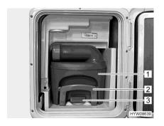
Fig. 141 Sewage tank (in the vehicle)
