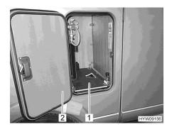
Fig. 80 Gas bottle compartment pull-out
