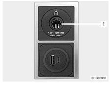
Fig. 77 12 V socket and USB ports
