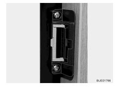
Fig. 123 Locking device (ventilation position)
