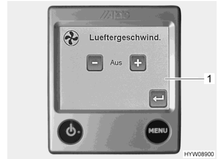
Fig. 130 Control (auxiliary fan)
