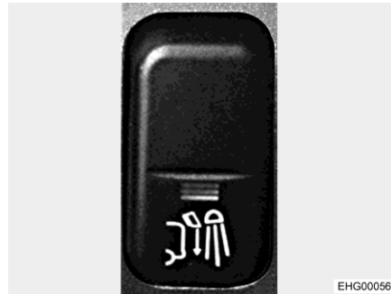
Fig. 26 Rocker switch (rear area lighting)
