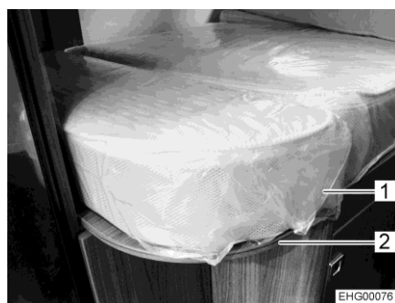
Fig. 81 Lying surface extension with additional cushion
