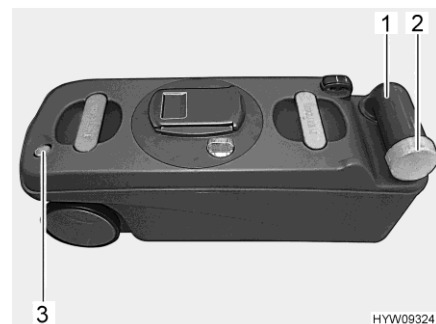
Fig. 171 Sewage tank (example)
