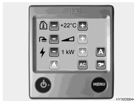
Fig. 124 Adjustment menu (operating unit)
