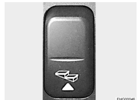
Fig. 10 Rocker switch for entrance step (dashboard)
