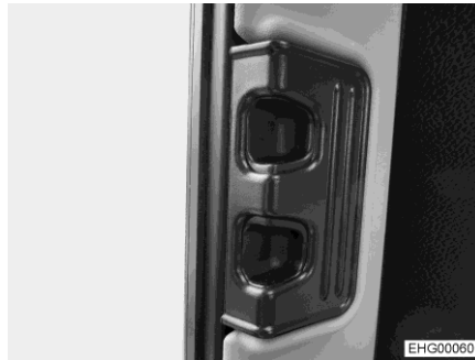
Fig. 45 Locking handle (front passenger's window)
