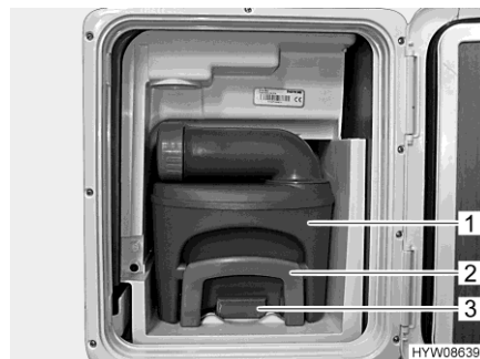
Fig. 170 Sewage tank (in the vehicle)
