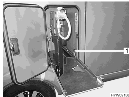
Fig. 91 Gas bottle compartment pull-out in changing position
