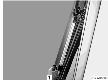
Fig. 42 Window support (hinged roof window)
