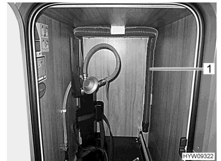
Fig. 160 Waste water hose (gas bottle compartment pull-out)
