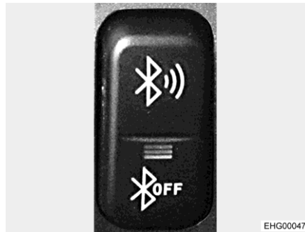
Fig. 96 Rocker button (Bluetooth connection)
