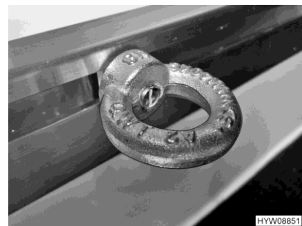
Fig. 7 Clamping eyelet (clamped)
