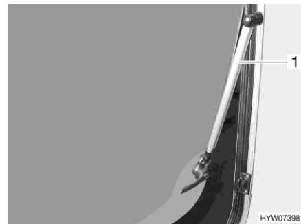
Fig. 39 Hinged window with automatic hinge
