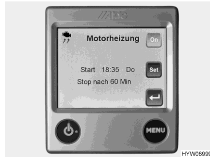
Fig. 127 Start menu (auxiliary circulating pump)
