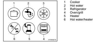
Fig. 81 Possible symbols for the gas isolator taps
