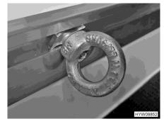
Fig. 4 Clamping eyelet (movable)
