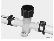
Fig. 126 Safety/drainage valve (Truma)
