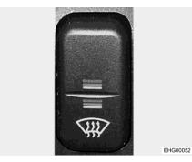
Fig. 9 Rocker switch (windscreen heater)
