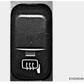
Fig. 17 Switch (electrically adjustable external mirrors)
