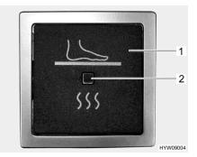
Fig. 113 Switch (electrical floor warming unit)
