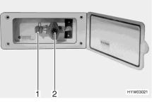
Fig. 83 External gas connection (gas isolator tap closed)
