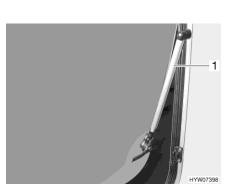
Fig. 41 Catch lever ("closed" position)
