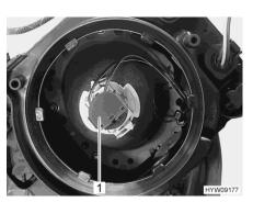
Fig. 150 Bulb (low beam/main beam)
