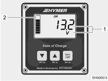
volts (V) 2 Display of state of charge (SoC)
