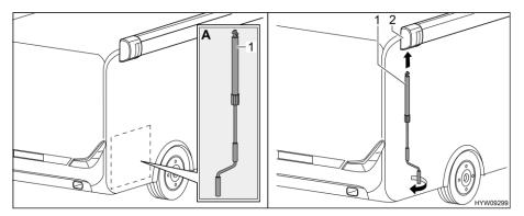
Fig. 29 Installing crank
