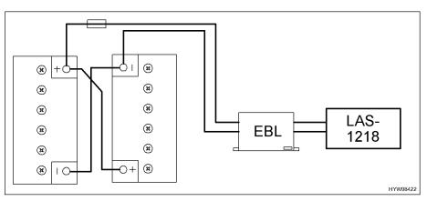
Fig. 92 Connecting auxiliary battery
