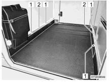
Fig. 3 Clamping eyelets (rear garage)
