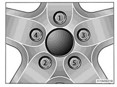
Fig. 160 Tightening the wheel nuts or wheel bolts cross-wise
