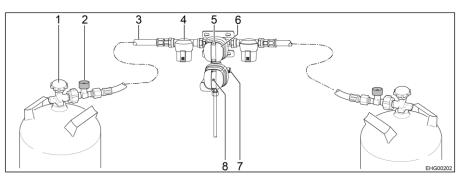
Fig. 87 Safety gas pressure regulating system DuoControl CS
