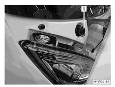
Fig. 22 Filler neck (washer fluid container)
