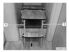
Fig. 78 Access ladder (folded out)
