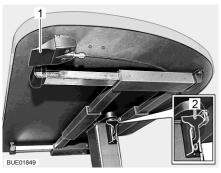
Fig. 55 Lift-off table with release button
