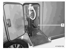
Fig. 86 Gas bottle compartment pull-out in changing position
