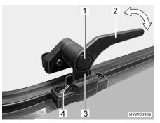
Fig. 43 Catch lever ("continuous ventilation" position)
