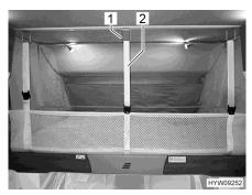
Fig. 63 Safety net (pull-down bed)
