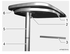
Fig. 58 Suspension table with separable support leg
