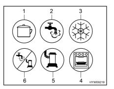
Fig. 105 Possible symbols for the gas isolator taps
