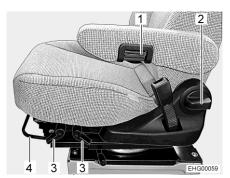
Fig. 14 Seat adjustment (Aguti GIS-Liner)
