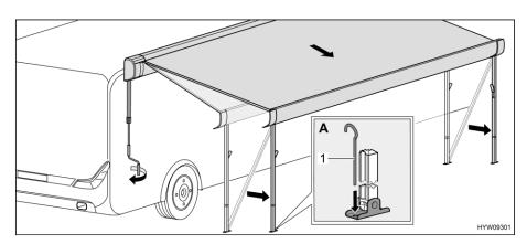
Fig. 31 Bringing awning into end position
