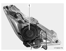
Fig. 149 Front headlight (rear side)
