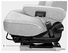
Fig. 52 Lever (turning the seat) (Aguti GIS-Liner)
