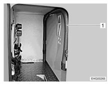
Fig. 130 Waste water hose (gas bottle compartment)
