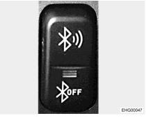
Fig. 91 Rocker button (Bluetooth connection)
