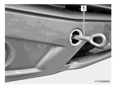
Fig. 25 Cover (mount of the towing eye)
