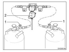
Fig. 10 Gas regulator (DuoControl CS)
