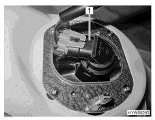
Fig. 152 Curve light/fog light (from below)
