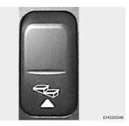
Fig. 7 Rocker switch for entrance step (entrance area)
