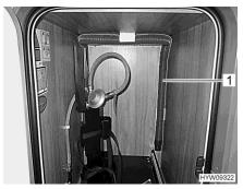
Fig. 131 Waste water hose (gas bottle compartment pull-out)
