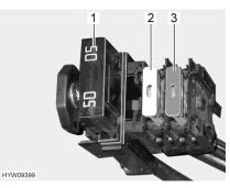
Fig. 99 Fuses (starter battery)
