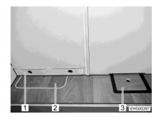
Fig. 142 Access to waste water tank at rear
