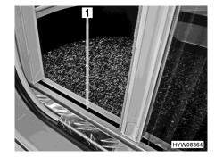
Fig. 19 Insect screen (bottom guide)
