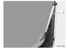
Fig. 22 Hinged window with automatic hinge
