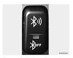
Fig. 71 Rocker button (Bluetooth connection)
