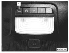
Fig. 7 Button for the call for breakdown assistance
