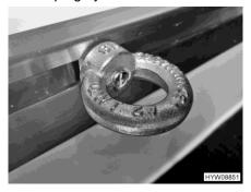
Fig. 1 Clamping eyelet (movable)
