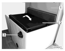
Fig. 11 Folding out the additional seat
