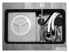
Fig. 106 Rotary handle (water tank)
