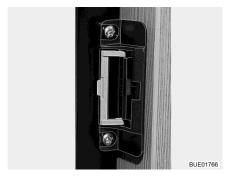
Fig. 102 Locking device (ventilation position)
