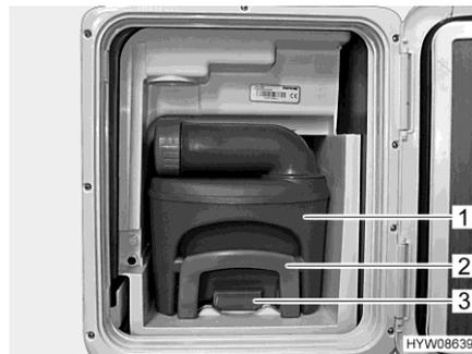
Fig. 137 Sewage tank (in the vehicle)
