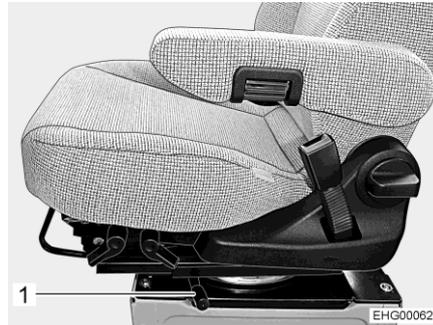
Fig. 52 Lever (turning the seat)
