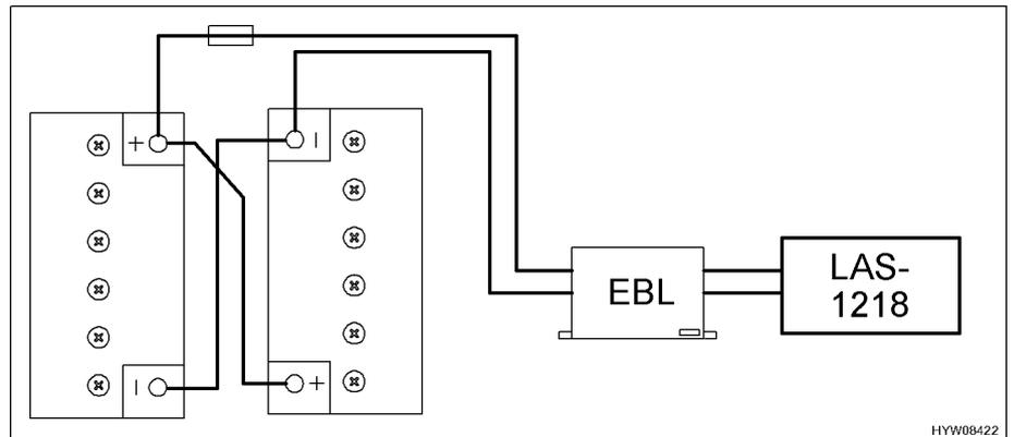
Fig. 92 Connecting auxiliary battery
