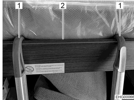
Fig. 64 Access ladder (pull-down bed)
