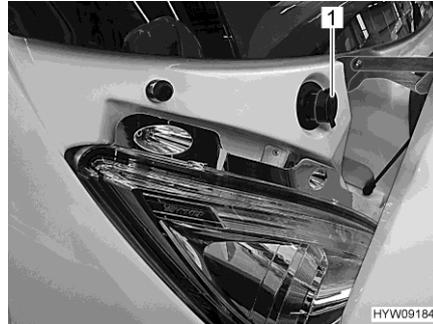
Fig. 22 Filler neck (washer fluid container)
