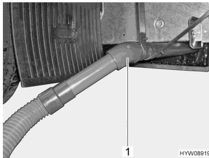
Fig. 132 Drain pipe with waste water hose
