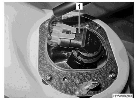
Fig. 152 Curve light/fog light (from below)
