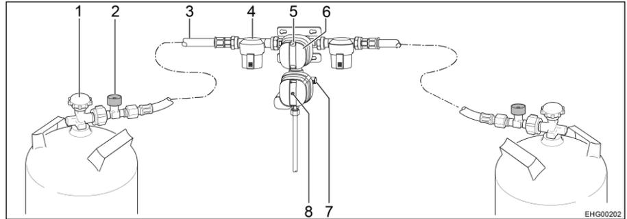
Fig. 87 Safety gas pressure regulating system DuoControl CS
