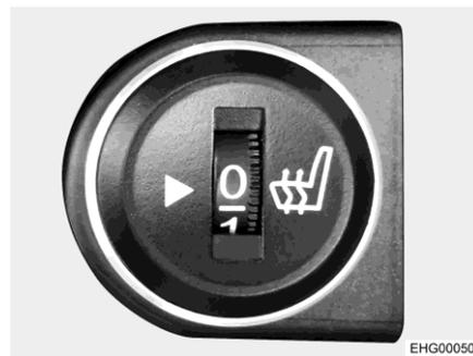
Fig. 15 Switch for seat heater
