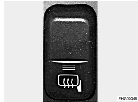
Fig. 18 Switch (mirror heater)
