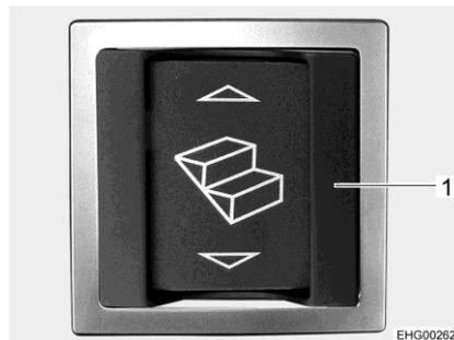
Fig. 7 Rocker switch for entrance step (entrance area)
