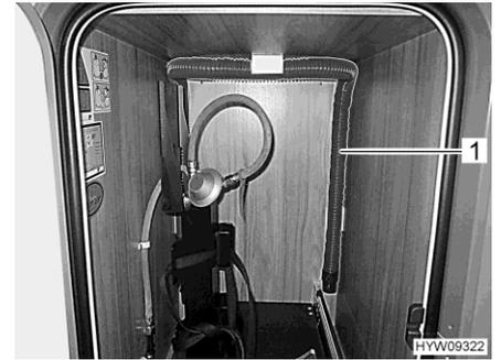
Fig. 131 Waste water hose (gas bottle compartment pull-out)
