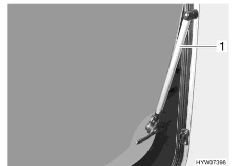
Fig. 42 Hinged window with automatic hinge
