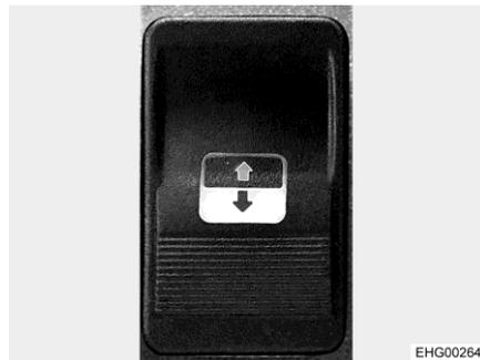
Fig. 16 Switch (electrical window winder in the driver's door)
