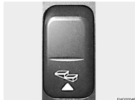
Fig. 8 Rocker switch for entrance step (dashboard)
