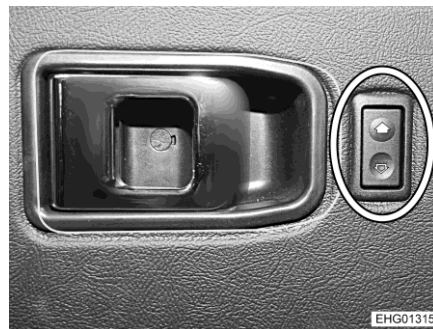
Fig. 31 Rocker switch (electrical window winder in the driver's door)
