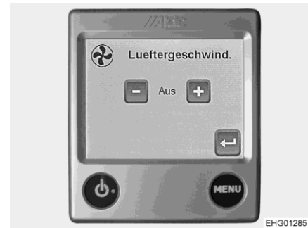
Fig. 179 Control (auxiliary fan)
