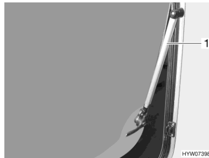
Fig. 62 Hinged window with automatic hinge
