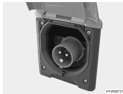
Fig. 149 230 V connection on the vehicle (CEE socket outlet)
