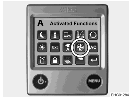
Fig. 178 Booster function (auxiliary fan)
