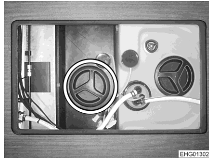
Fig. 220 Cleaning opening (waste water tank)
