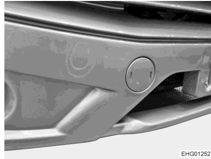
Fig. 40 Cover (mount of the towing eye)
