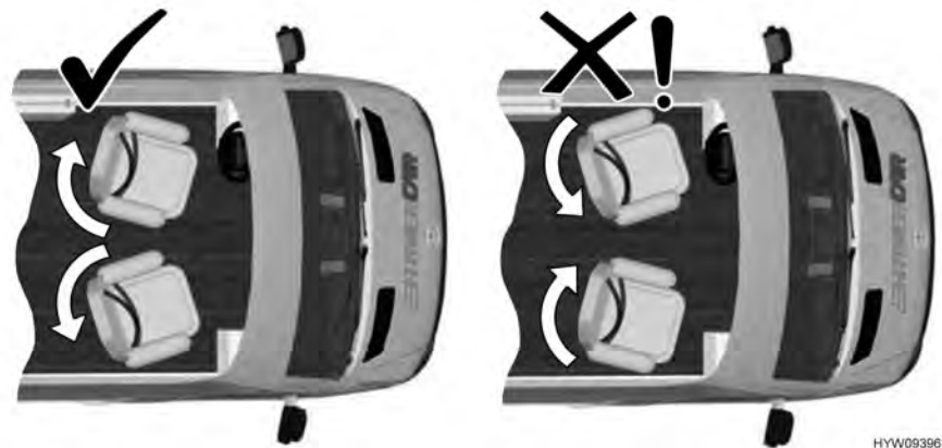
Fig. 41 Observe the direction of rotation of driver's/front passenger's seat
