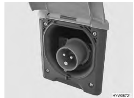
Fig. 66 240 V connection on the vehicle (CEE socket outlet)
