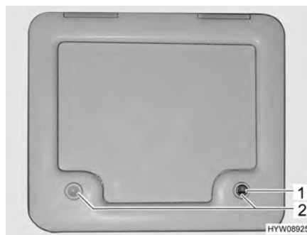
Fig. 110 Flap (sewage tank)
