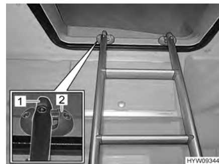
Fig. 34 Access ladder (attached)
