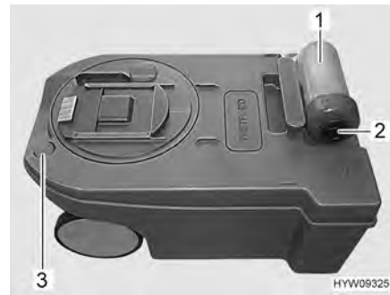
Fig. 114 Sewage tank (alternative)
