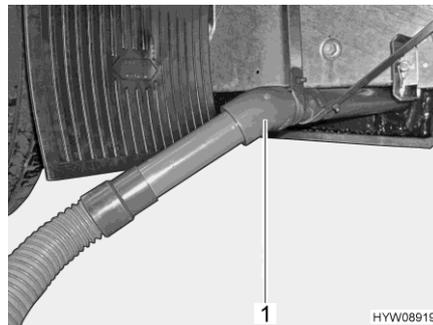
Fig. 144 Drain pipe with waste water hose
