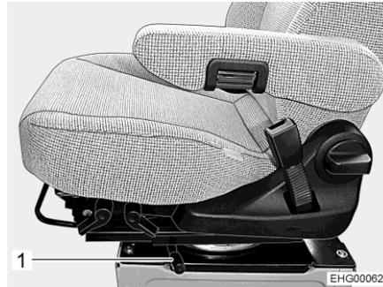
Fig. 58 Lever (turning the seat)
