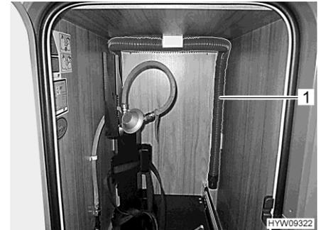
Fig. 143 Waste water hose (gas bottle compartment pull-out)
