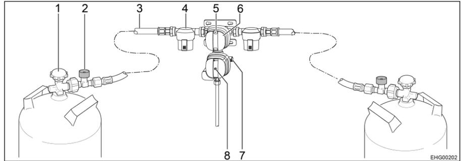
Fig. 94 Safety gas pressure regulating system DuoControl CS
