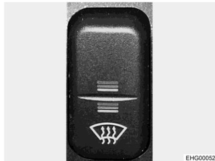
Fig. 11 Rocker switch (windscreen heater)
