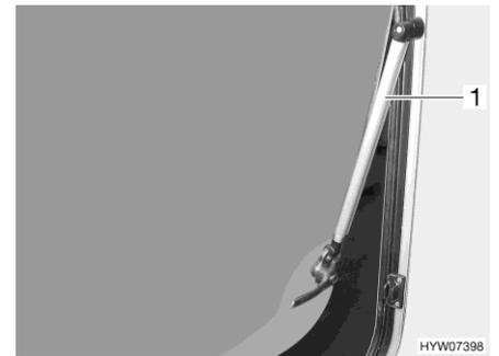
Fig. 45 Hinged window with automatic hinge
