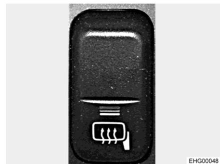
Fig. 21 Switch (mirror heater)
