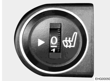
Fig. 18 Switch for seat heater
