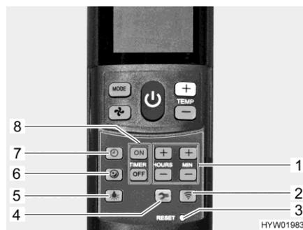
Fig. 123 Remote control with setting buttons (air conditioning unit)
