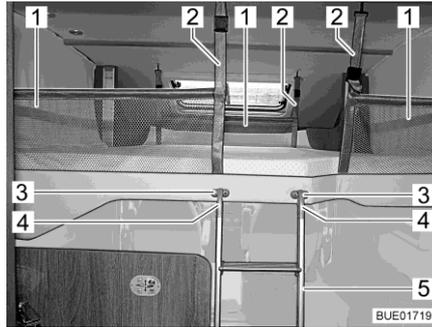
Fig. 74 Pull-down bed complete with applied safety net
