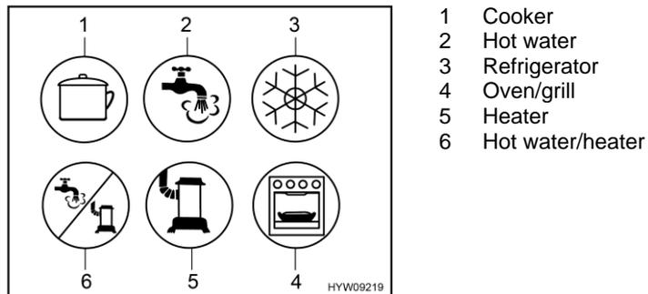
Fig. 112 Possible symbols for the gas isolator taps
