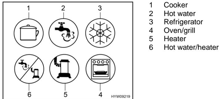
Fig. 88 Possible symbols for the gas isolator taps
