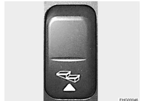
Fig. 10 Rocker switch for entrance step (dashboard)
