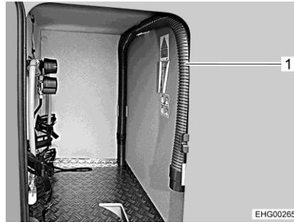
Fig. 142 Waste water hose (gas bottle compartment)
