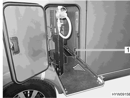
Fig. 93 Gas bottle compartment pull-out in changing position
