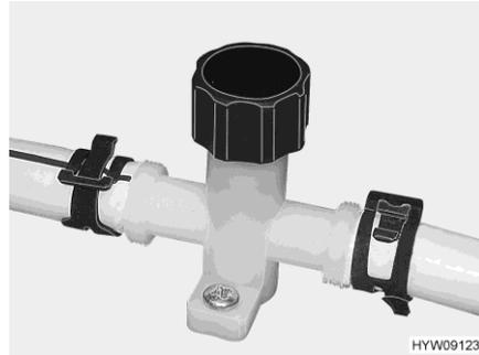
Fig. 151 Drain cock (water pipe)
