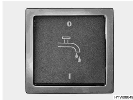
Fig. 137 Switch (water pump)
