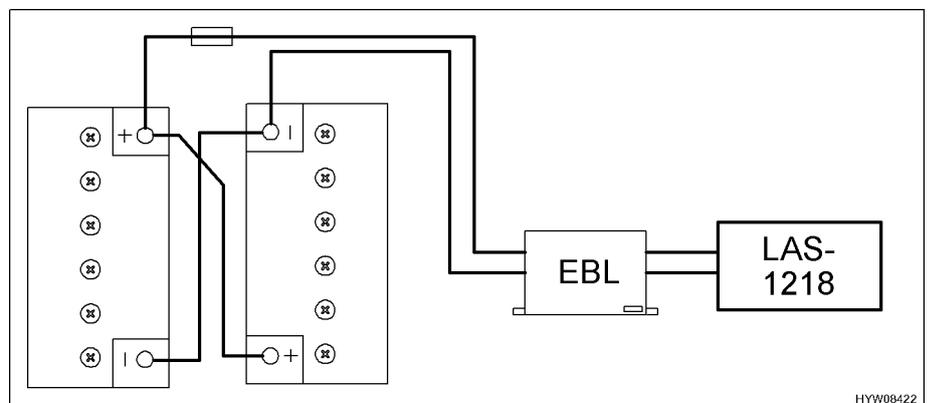
Fig. 101 Connecting auxiliary battery
