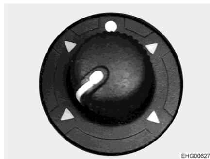
Fig. 20 Switch (electrically adjustable external mirrors)
