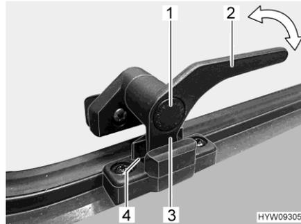
Fig. 46 Catch lever ("continuous ventilation" position)
