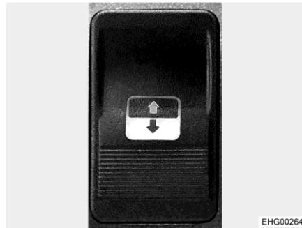
Fig. 19 Switch (electrical window winder in the driver's door)
