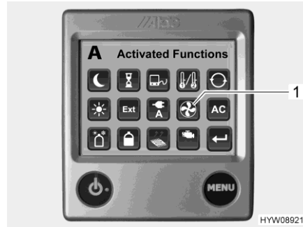
Fig. 183 Activated functions (auxiliary fan)
