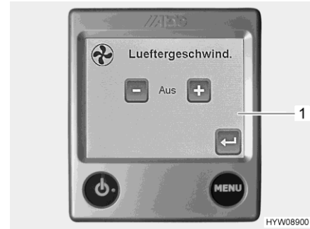
Fig. 184 Control (auxiliary fan)
