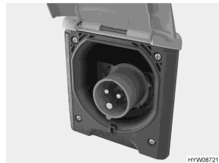
Fig. 153 230 V connection on the vehicle (CEE socket outlet)
