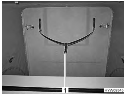
Fig. 37 Auxiliary strap (elevating roof)
