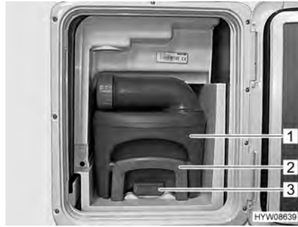
Fig. 111 Sewage tank (in the vehicle)
