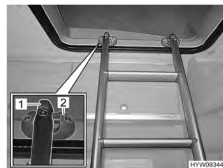
Fig. 34 Access ladder (attached)
