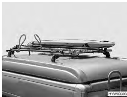
Fig. 1 Elevating roof with roof rack
