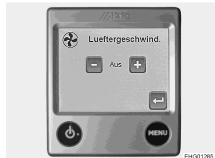
Afb. 179 Besturing (extra ventilator)
