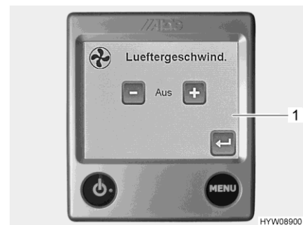
Afb. 166 Besturing (extra ventilator)
