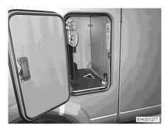
Fig. 128 Gas bottle compartment pull-out
