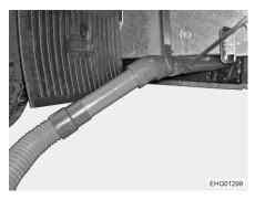
Fig. 207 Drain pipe with waste water hose
