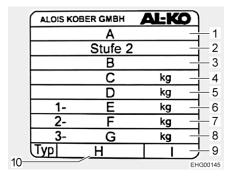
Fig. 238 Vehicle identification plate on the chassis
