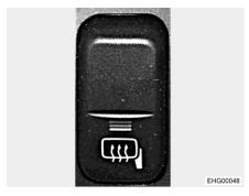
Fig. 36 Rocker switch (mirror heater)
