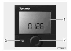
Fig. 164 Control unit (hot-air heater and boiler)
