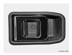
Fig. 56 Door lock (driver's door, inside)
