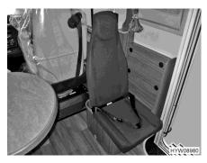
Fig. 30 Attachable seat unfolded
