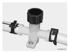
Fig. 162 Drain cock (water pipe)
