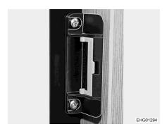
Fig. 196 Locking device (normal position)
