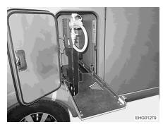
Fig. 130 Gas bottle compartment pull-out in changing position
