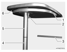
Fig. 92 Suspension table with separable support leg
