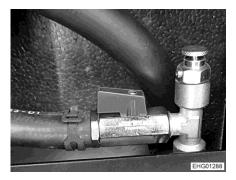
Fig. 182 Spherical valve (opened)
