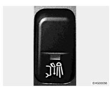
Fig. 45 Rocker switch (rear area lighting)
