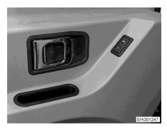
Fig. 34 Rocker switch (electrical window winder in the driver's door)
