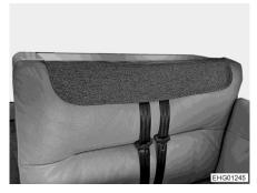
Fig. 16 Seat belt cover attached
