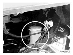
Fig. 40 Filler neck (washer fluid container)
