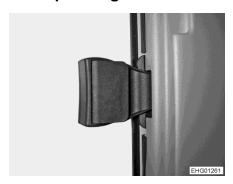
Fig. 62 Handle for opening the front passenger's window
