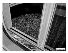
Fig. 59 Insect screen (bottom guide)
