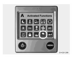
Fig. 180 Engine heater function (auxiliary fan)
