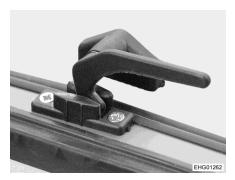
Fig. 68 Catch lever ("continuous ventilation" position)
