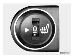
Fig. 23 Switch for seat heater
