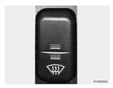
Fig. 11 Rocker switch (windscreen heater)
