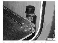
Fig. 129 Knob with locking device
