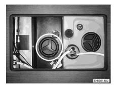
Fig. 220 Cleaning opening (waste water tank)
