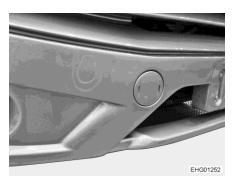
Fig. 43 Cover (mount of the towing eye)
