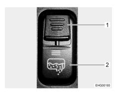
Fig. 204 Rocker switch (waste water drainage)
