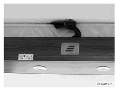
Fig. 100 Retaining belt
