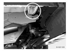
Fig. 240 Front axle mount
