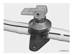
Fig. 172 Drain cock (water pipe)
