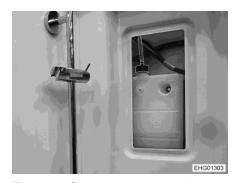
Fig. 222 Compensator reservoir (hot-water heater)
