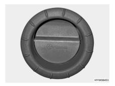
Fig. 157 Air outlet nozzle (hot-air heater)
