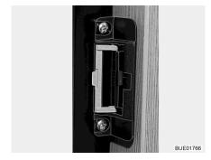
Fig. 197 Locking device (ventilation position)
