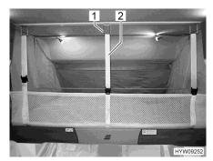
Fig. 101 Safety net (pull-down bed)
