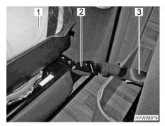
Fig. 29 Belt lock for attachable seat
