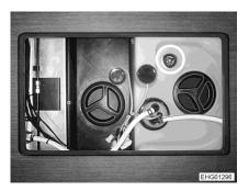
Fig. 203 Rotary handle (water drainage)
