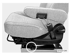
Fig. 81 Lever for turning the seat
