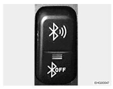
Fig. 136 Rocker switch (Bluetooth connection)
