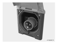
Fig. 147 230 V connection on the vehicle (CEE socket outlet)
