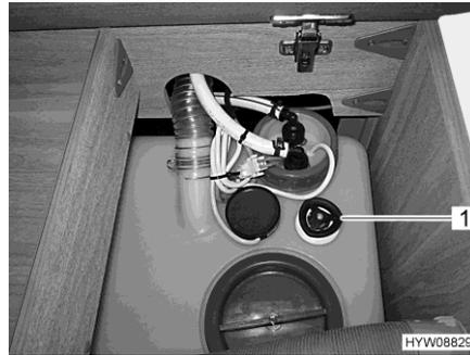
Fig. 101 Rotary handle (water drainage)
