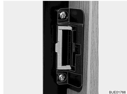
Fig. 94 Locking device (ventilation position)
