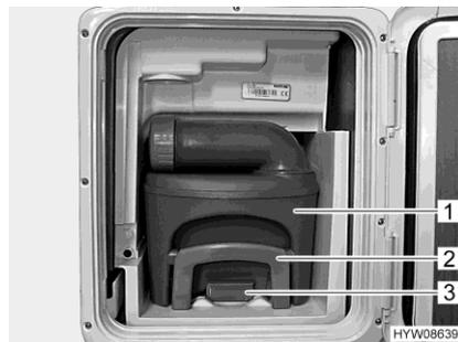
Fig. 113 Sewage tank (in the vehicle)
