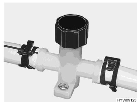
Fig. 88 Drain cock (water pipe)
