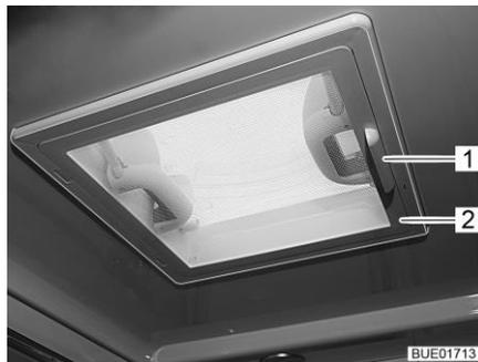
Fig. 25 Skylight with snap latch
