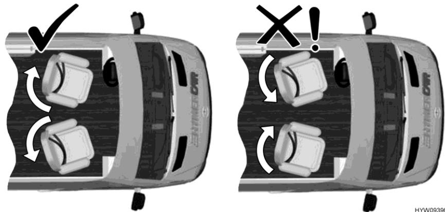
Fig. 44 Observe the direction of rotation of driver's/front passenger's seat
