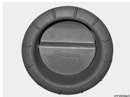
Fig. 76 Air outlet nozzle (hot-air heater)
