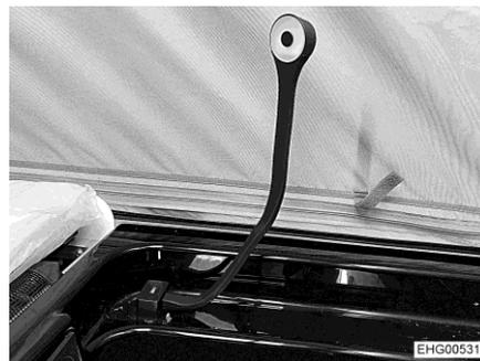
Fig. 39 Goose neck lamp, operating position
