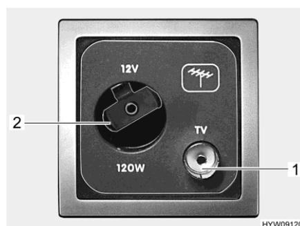
Fig. 59 Sockets (external satellite antenna)
