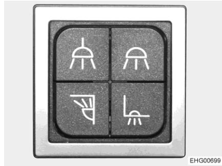
Fig. 73 Multi-light switch (example)
