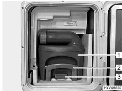
Fig. 141 Sewage tank (in the vehicle)
