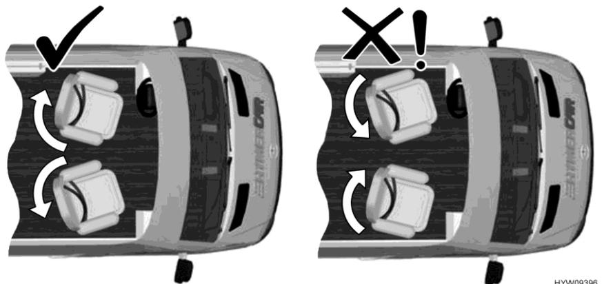
Fig. 49 Observe the direction of rotation of driver's/front passenger's seat
