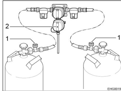
Fig. 8 Gas regulator (DuoControl CS)
