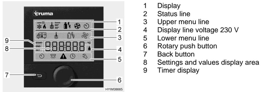
Fig. 105 Operating unit with displays
