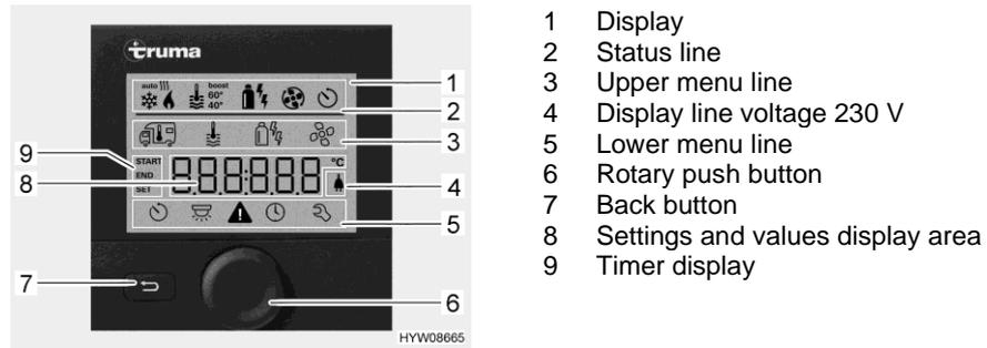
Fig. 110 Operating unit with displays
