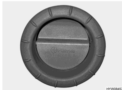
Fig. 103 Air outlet nozzle (hot-air heater)
