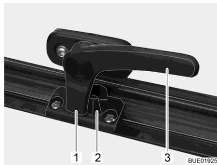
Fig. 19 Catch lever ("closed" position)
