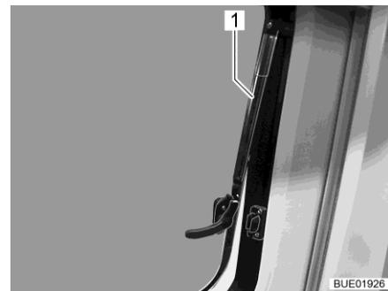
Fig. 20 Hinged window with automatic hinge
