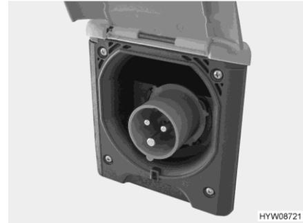
Fig. 97 230 V connection on the vehicle (CEE socket outlet)
