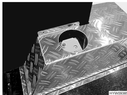
Fig. 134 Electrical waste water valve (rear garage)
