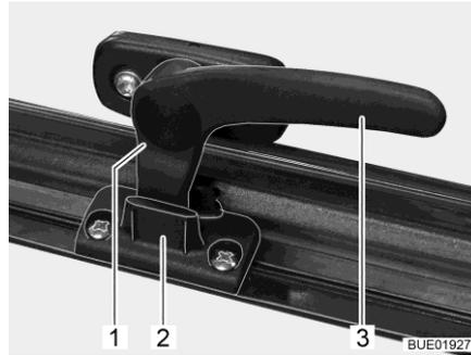
Fig. 21 Catch lever ("continuous ventilation" position)
