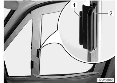
Fig. 26 Roman shade (driver's / front passenger's window, Mercedes-Benz)
