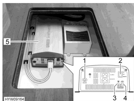
Fig. 94 AC converter (exemplary illustration)
