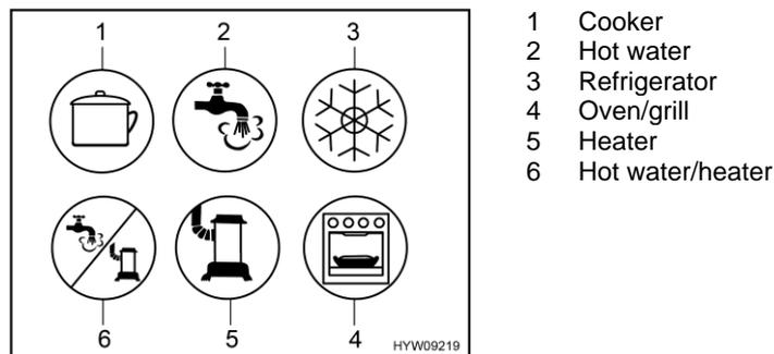
Fig. 102 Possible symbols for the gas isolator taps
