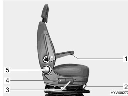
Fig. 10 Operating controls on seat (Fiat as example)
