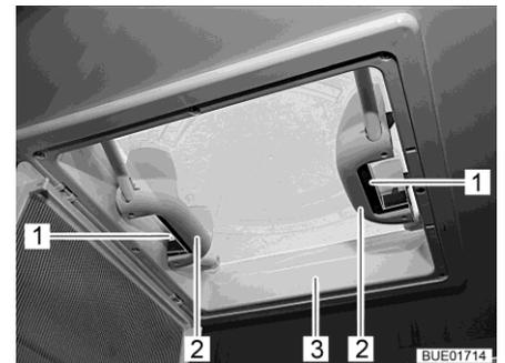
Fig. 31 Handles with snap latches
