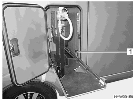
Fig. 82 Gas bottle compartment pull-out in changing position
