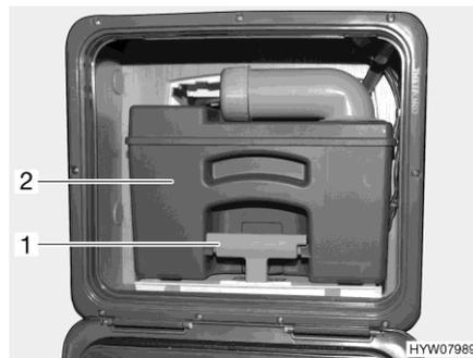
Fig. 143 Sewage tank (in the vehicle) (alternative)
