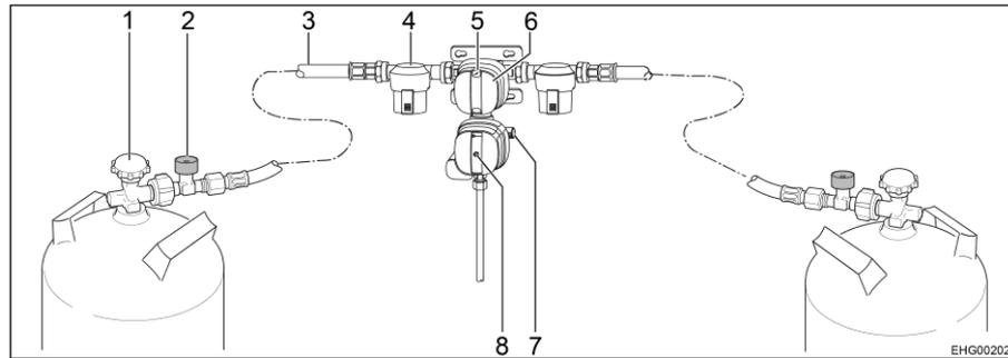
Fig. 65 Safety gas pressure regulating system DuoControl CS
