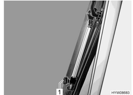
Fig. 25 Window support (hinged roof window)
