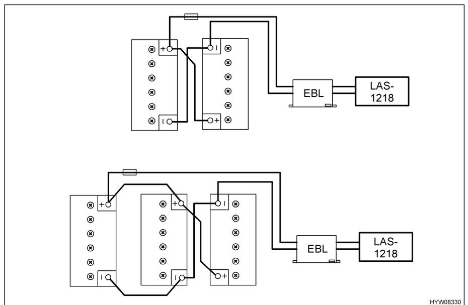
Fig. 72 Connecting auxiliary battery
