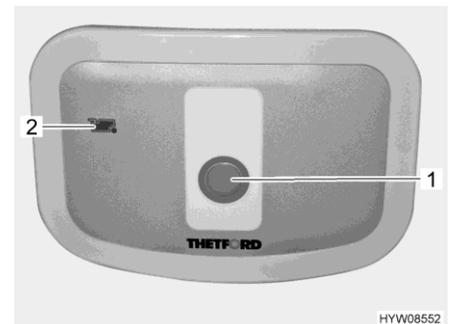
Fig. 111 Flush button/indicator lamp (Thetford toilet)
