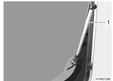
Fig. 22 Hinged window with automatic hinge
