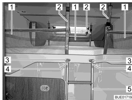
Fig. 52 Pull-down bed complete with applied safety net
