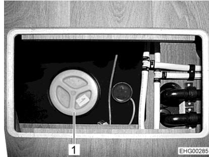
Fig. 118 Cleaning opening (waste water tank)
