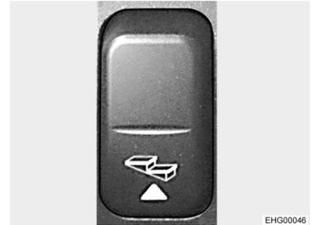
Fig. 5 Rocker switch for entrance step (dashboard)
