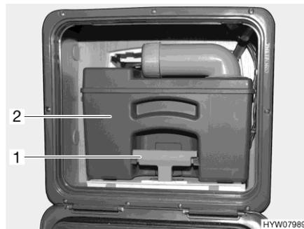
Fig. 113 Sewage tank (in the vehicle)
