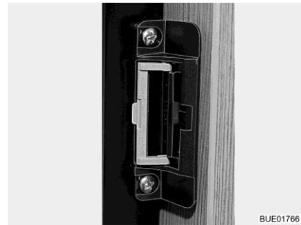
Fig. 102 Locking device (ventilation position)
