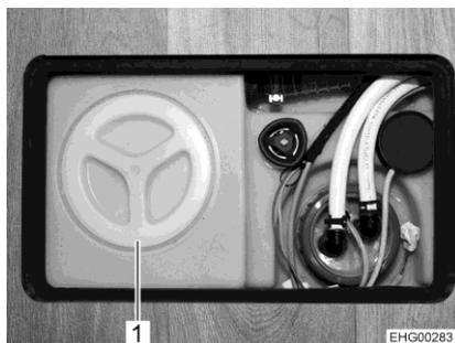
Fig. 117 Cleaning opening (water tank)
