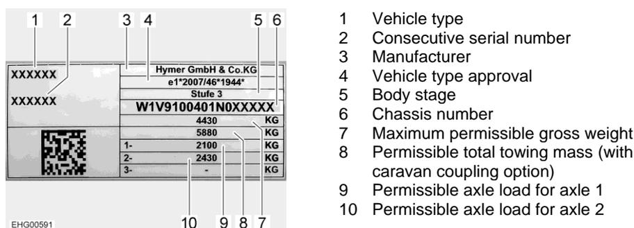
Fig. 128 Vehicle identification plate
