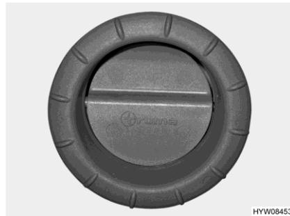
Fig. 86 Air outlet nozzle (hot-air heater)
