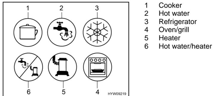
Fig. 85 Possible symbols for the gas isolator taps
