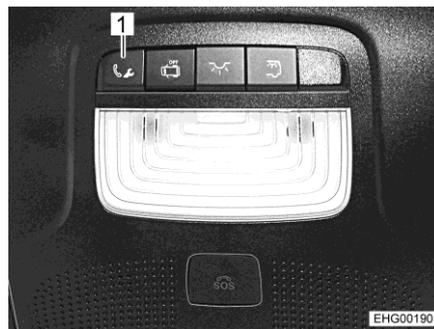
Fig. 7 Button for the call for breakdown assistance
