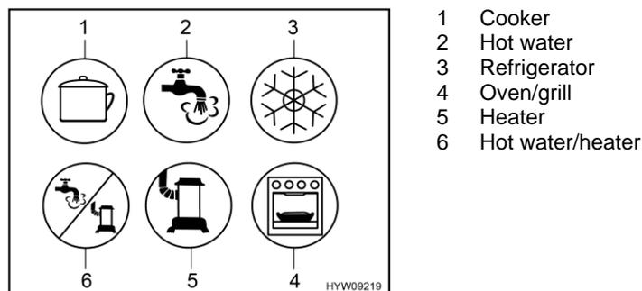
Fig. 62 Possible symbols for the gas isolator taps
