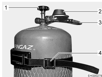
Fig. 68 Camping gas bottle connection
