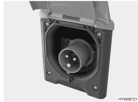
Fig. 78 230 V connection on the vehicle (CEE socket outlet)
