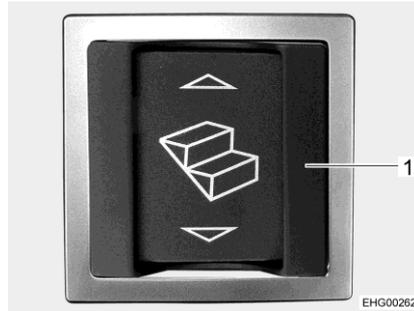
Fig. 4 Rocker switch for entrance step (entrance area)
