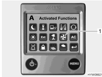
Fig. 129 Activated functions (auxiliary fan)
