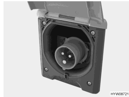
Fig. 107 230 V connection on the vehicle (CEE socket outlet)
