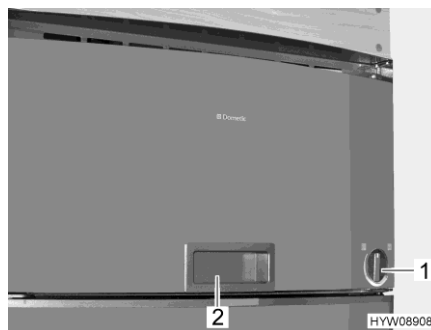
Fig. 143 Gas oven (integrated on refrigerator)
