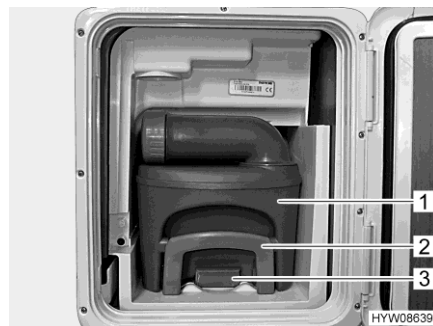
Fig. 170 Sewage tank (in the vehicle)
