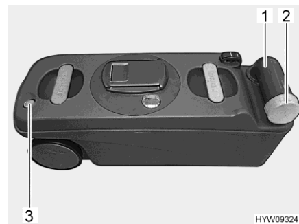
Fig. 171 Sewage tank (example)
