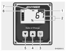
Fig. 102 Display panel (display of state of charge)
