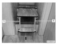
Fig. 85 Access ladder (folded out)
