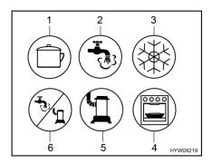
Fig. 88 Possible symbols for the gas isolator taps
