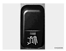
Fig. 30 Rocker switch (rear area lighting)
