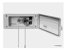
Fig. 90 External gas connection (gas isolator tap closed)
