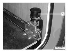
Fig. 92 Knob with locking device
