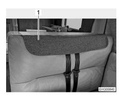
Fig. 13 Seat belt cover attached
