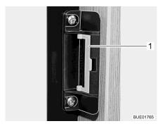
Fig. 135 Locking device (normal position)
