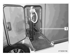
Fig. 93 Gas bottle compartment pull-out in changing position
