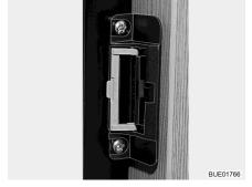
Fig. 136 Locking device (ventilation position)
