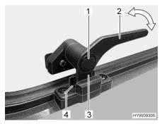
Fig. 46 Catch lever ("continuous ventilation" position)
