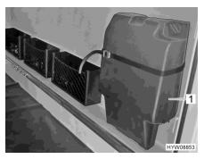
Fig. 171 Storage box (on-board tool set)
