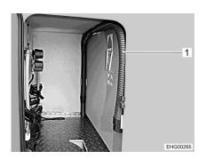
Fig. 142 Waste water hose (gas bottle compartment)
