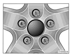
Fig. 169 Tightening the wheel nuts or wheel bolts cross-wise
