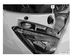
Fig. 25 Filler neck (washer fluid container)
