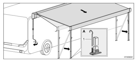
Fig. 34 Bringing awning into end position
