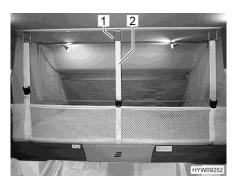
Fig. 71 Safety net (pull-down bed)
