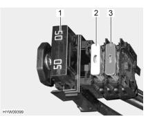
Fig. 108 Fuses (starter battery)
