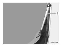
Fig. 45 Hinged window with automatic hinge
