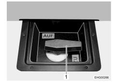
Fig. 145 Operating lever (waste water tank)
