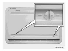
Fig. 132 Refrigerator ventilation grill
