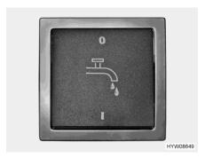
Fig. 137 Switch (water pump)
