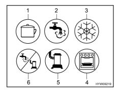
Fig. 112 Possible symbols for the gas isolator taps
