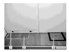
Fig. 154 Access to waste water tank at rear
