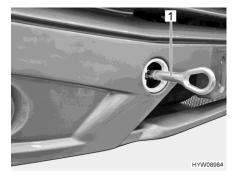
Fig. 29 Towing eye (mounted)
