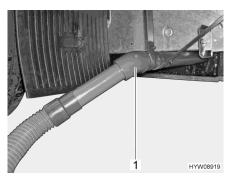
Fig. 144 Drain pipe with waste water
