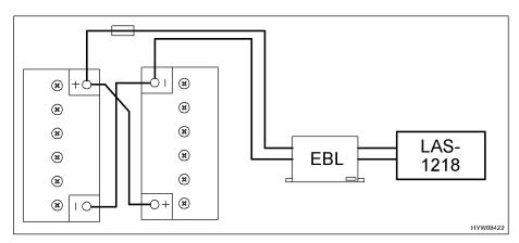
Fig. 101 Connecting auxiliary battery
