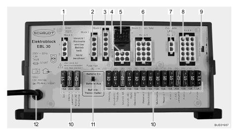
Fig. 104 Transformer/rectifier (EBL 30)
