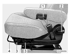
Fig. 17 Seat adjustment (Aguti GIS-Liner)
