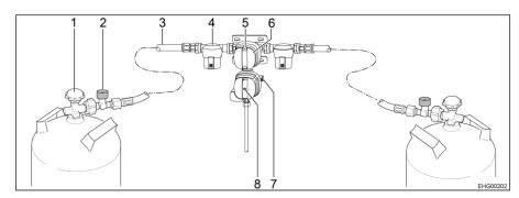
Fig. 94 Safety gas pressure regulating system DuoControl CS
