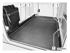
Fig. 5 Clamping eyelets (rear garage)
