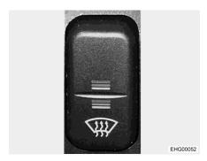
Fig. 11 Rocker switch (windscreen heater)
