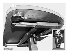
Fig. 63 Lift-off table with release button
