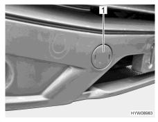
Fig. 28 Cover (mount of the towing
