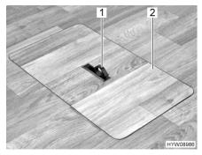
Fig. 60 Floor storage compartment cover (handle swung out)
