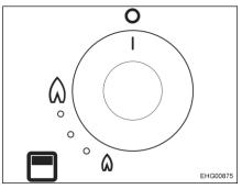
Fig. 129 Control knob for gas grill
