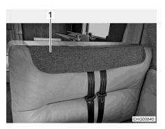
Fig. 61 Seat belt cover attached
