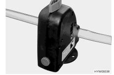
Fig. 151 Drain cock (water pipe)
