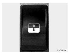
Fig. 19 Switch (electrical window winder in the driver's door)
