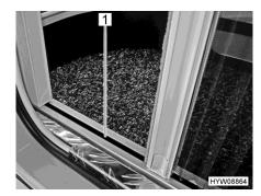
Fig. 41 Insect screen (bottom guide)
