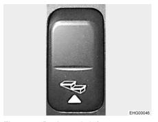
Fig. 10 Rocker switch for entrance step (dashboard)
