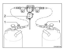
Fig. 12 Gas regulator (DuoControl CS)
