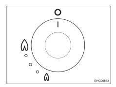
Fig. 127 Control knob for gas burn-
