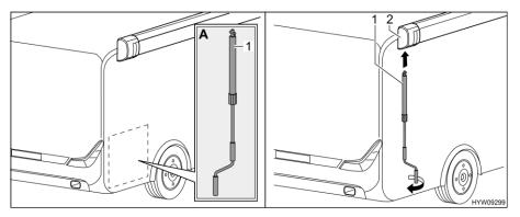
Fig. 32 Installing crank
