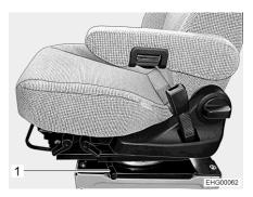
Fig. 58 Lever (turning the seat) (Aguti GIS-Liner)
