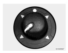
Fig. 20 Switch (electrically adjustable external mirrors)
