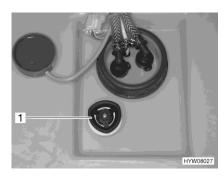
Fig. 141 Rotary handle (water tank)
