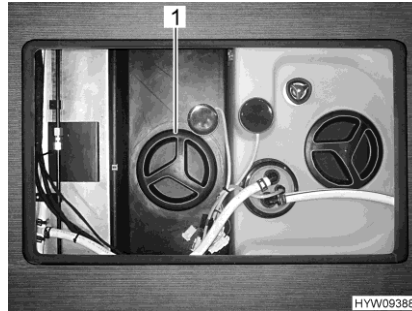
Afb. 221 Reinigingsopening (afvalwatertank)
