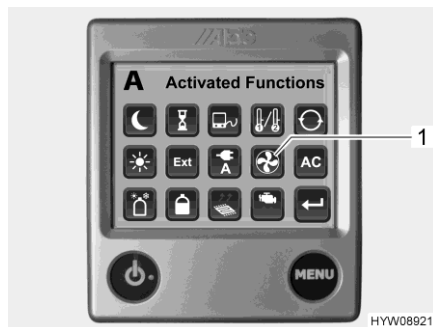
Fig. 178 Activated functions (auxiliary fan)
