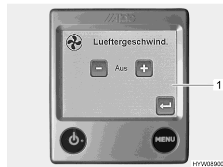
Fig. 179 Control (auxiliary fan)
