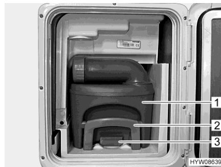
Fig. 215 Sewage tank (in the vehicle)
