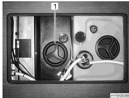
Fig. 221 Cleaning opening (waste water tank)
