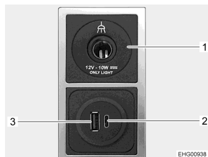
Fig. 98 Combination socket 12 V/USB
