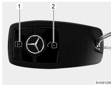
Fig. 53 Remote control for central locking system
