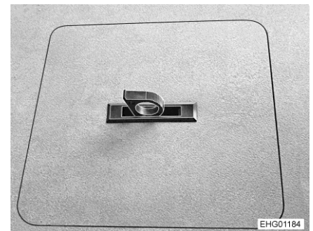
Fig. 72 Service cover (handle swivelled out)
