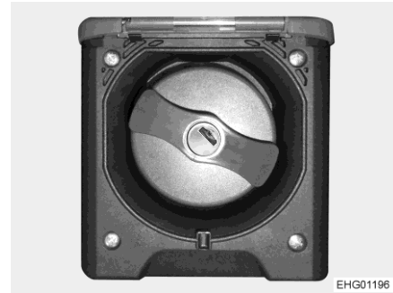
Fig. 125 Drinking water filler neck cap
