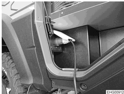
Fig. 105 230 V connection on the vehicle (CEE socket outlet)
