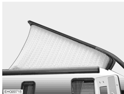
Fig. 39 Sleeping roof, open
