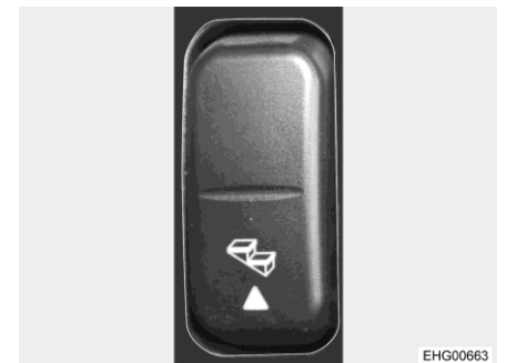
Fig. 5 Rocker button for entrance step (dashboard)
