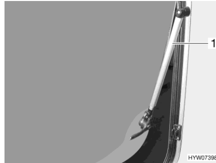
Fig. 60 Hinged window with automatic hinge
