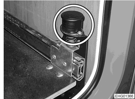
Fig. 92 Knob with locking device
