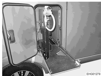
Fig. 93 Gas bottle compartment pull-out in changing position
