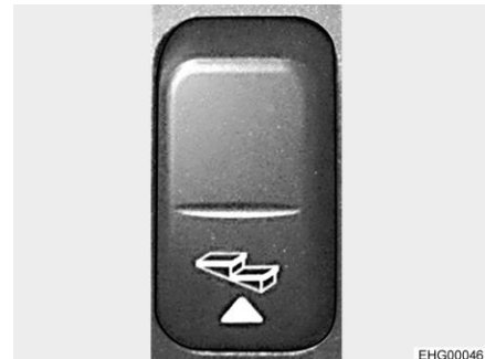
Fig. 11 Rocker button for entrance step (switch panel)
