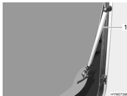
Fig. 42 Hinged window with automatic hinge
