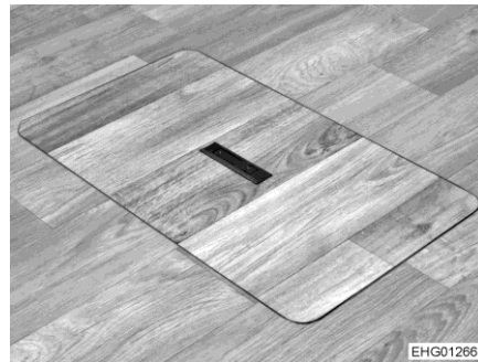
Fig. 61 Service cover (handle recessed)
