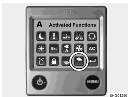
Fig. 125 Engine heater function (auxiliary fan)
