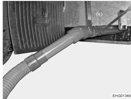
Fig. 148 Drain pipe with waste water hose
