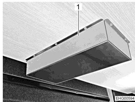
Fig. 115 Housing for the adjustment motor
