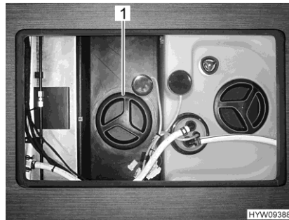
Fig. 226 Cleaning opening (waste water tank)
