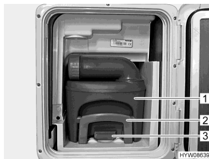
Fig. 220 Sewage tank (in the vehicle)
