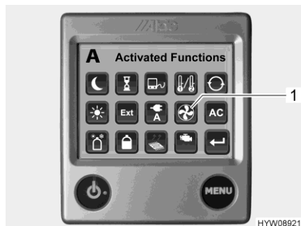
Fig. 178 Activated functions (auxiliary fan)
