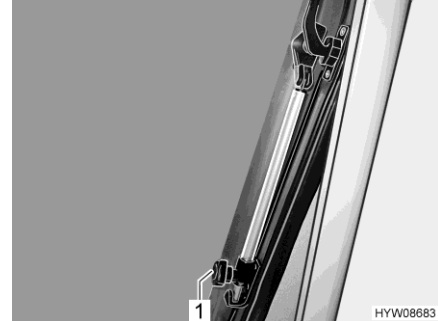
Fig. 67 Window support (hinged roof window)
