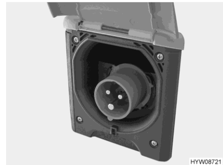
Fig. 151 230 V connection on the vehicle (CEE socket outlet)
