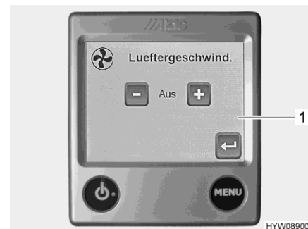
Fig. 179 Control (auxiliary fan)
